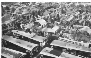
IN VIEW, MIDDLE: Wings and motor sections of 4-0-4 start movement to final assembly.
